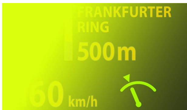
HUD image showing excessive heat or incidental light
